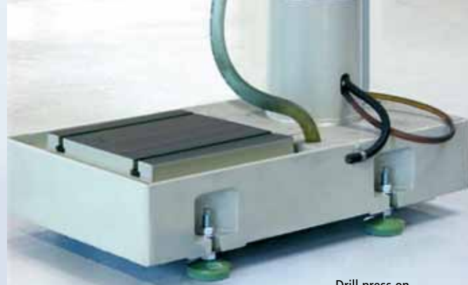
Drill press on leveling elements
