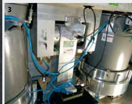
Illustr. 2: Experimentation area with 4.2 m of clearance and acoustic insulating materials (supplied and installed by BILZ). Source: Binnig and Rohrer Nanotechnology Centre (IBM Research – Zurich) Illustr. 3: AIS™ active vibration isolation from BILZ, which suspends the 75-tonne foundation block, with glass-fibre plastic reinforcement, on an air cushion. Source: Binnig and Rohrer Nanotechnology Centre (IBM Research – Zurich)
