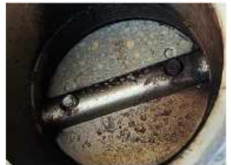
Intake valve coke deposits view
